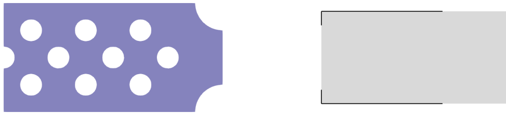
Fig. 4: Left: initial shape for optimization algorithm. Right: level set function constraint set \Sigma \subset \partial \widehat{\mathcal{D}} denoted by solid lines.
